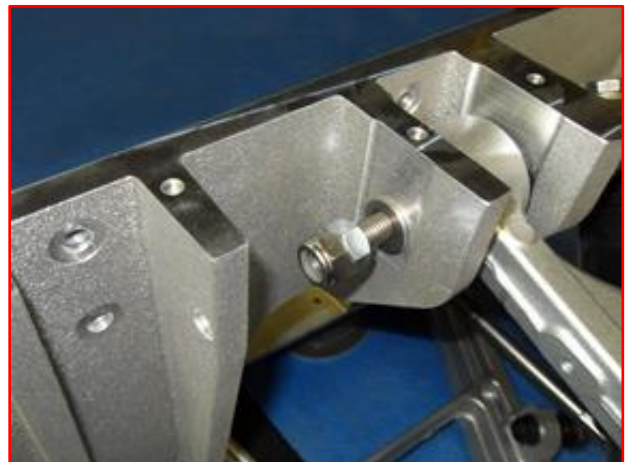
The front 12mm stud with two nuts.
